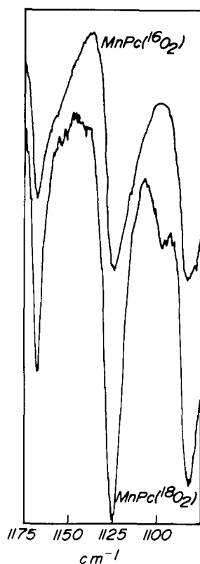
Figure 1. The infrared spectra of (O 2 )MnPc incorporating oxygen-16 and oxygen-18 in the region 1075-1175 cm -1 (Nujol mull).
